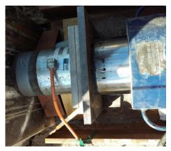
Lateral load test jack and load cell
