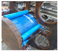
O-Cell and bearing plate assembly with reduced diameter bottom plate
